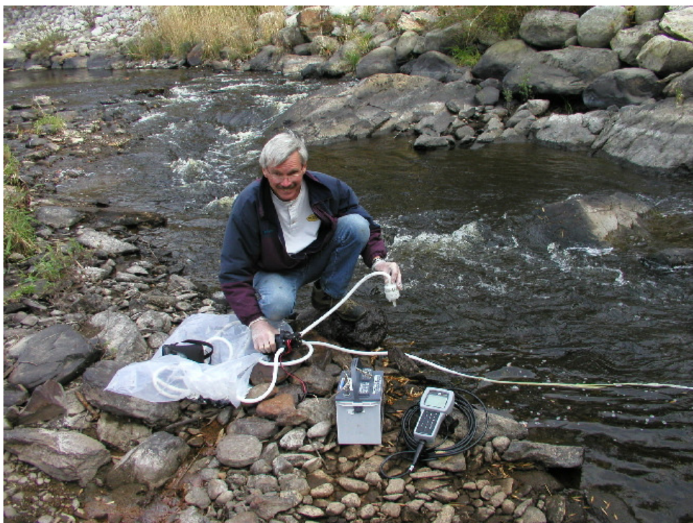
Photograph 2. Use of the continuous pumping system to collect water samples from a shallow stream. The inlet end of the tubing (out of picture) is screened and weighted. Capsule filter is shown installed on the discharge line from the pump.
