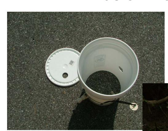
Intended as a device to isolate a section of near-bank sediment from continuous "flushing" by upstream surface water, i.e., a simplified benthic flux chamber
