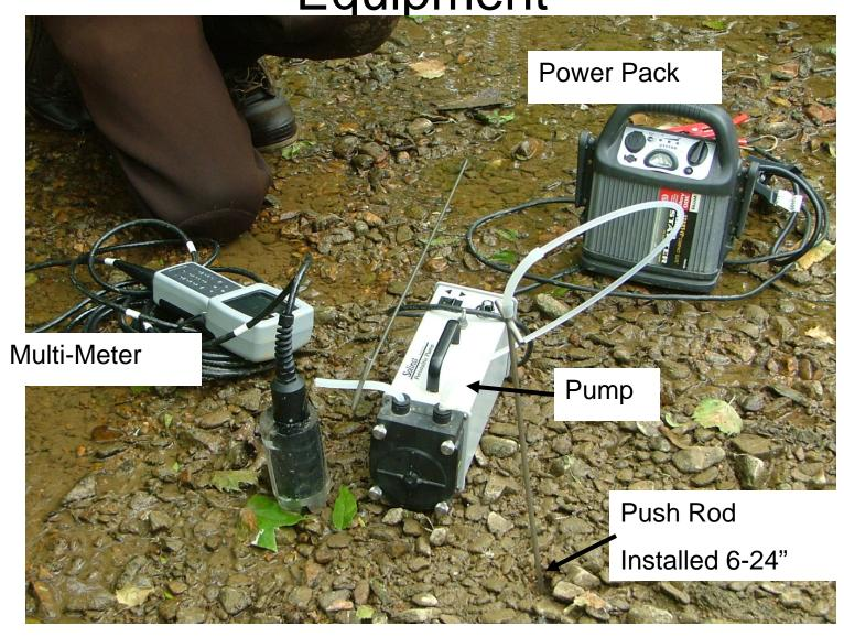
Also measure water level in manometer relative to river water level
