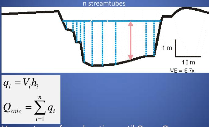
Vary water surface elevation until Q<sub>calc</sub> = Q<sub>measured</sub>
