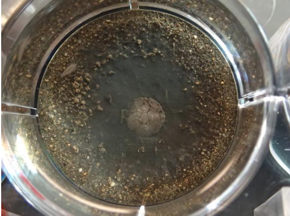
Figure 5. Close-up photograph of a leaf disc partially covered with Sedimite® at the end of a 10-day assay. Normal amphipod bioturbation of sediments caused Sedimite® to cover the sediment surfaces and often the leaf disc.
