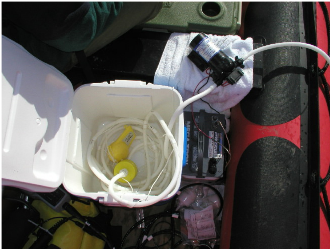
Photograph 1. Use of clean cooler to protect sample inlet line and hydro weight from contamination when sampling from a boat in deeper water. Round yellow object on end of C-flex tubing is plastic screen to prevent end of inlet line from touching sediment or sucking in algae or other debris. Hydro weight (yellow sphere with fin) is typically only required where current is very swift ( >0.5 m/s) and is tethered a foot or more below the sample inlet.
