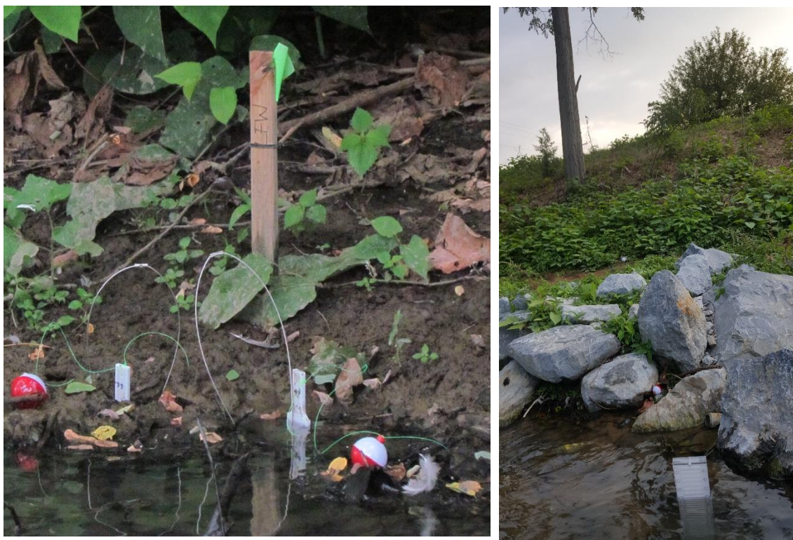
Figure 21 Bank location L3 DGT paddle profiler deployment during baseline condition July 2015 (left) and August 2017(right) sampling. Notice the differences in L3 location caused by stabilization effort implementation, as well as the deployment of a dialysis membrane at the L3 location during August 2017 sampling
