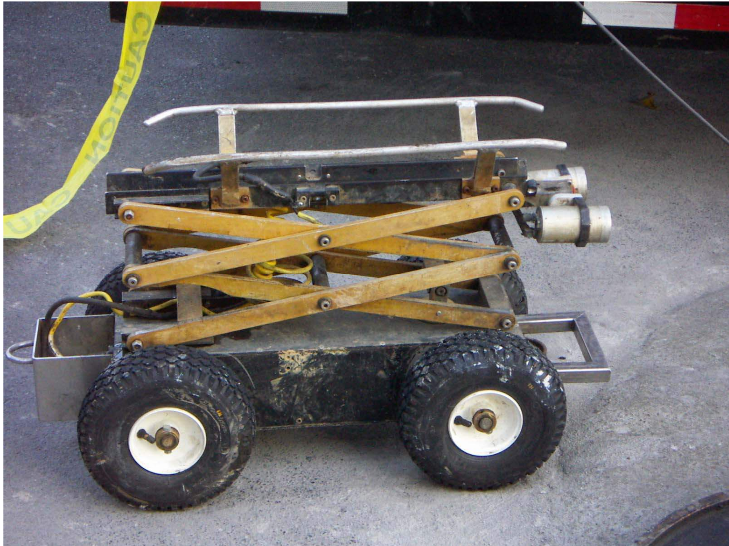
The tractor for pipes 24" and larger
