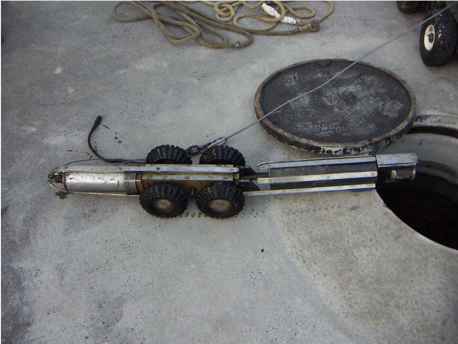
The camera for pipes 18" and smaller
